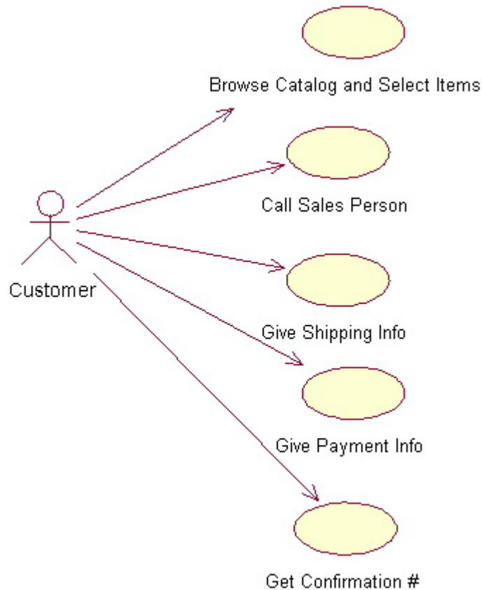
This example shows the customer as a actor because the customer is using the ordering system. The diagram takes the simple steps listed above and shows them as actions the customer might perform. The salesperson could also be included in this use case diagram because the salesperson is also interacting with the ordering system.
