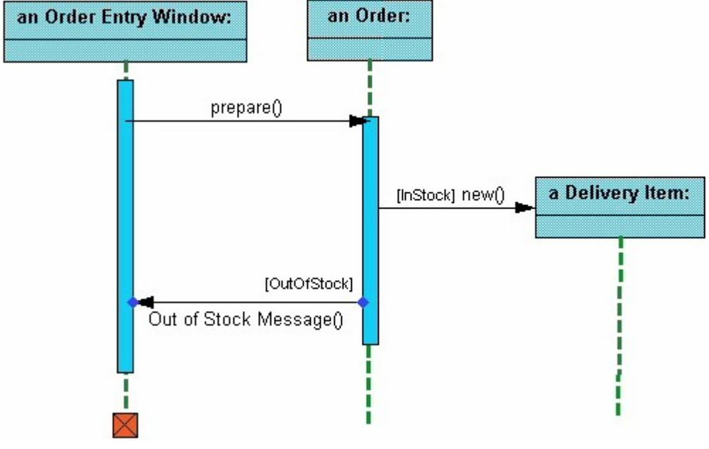
This simple diagram shows the sequence that messages are passed between objects to complete a use case for ordering an item.
