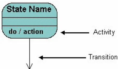
All state diagrams begin with an initial state of the object. This is the state of the object when it is created. After the initial state the object begins changing states. Conditions based on the activities can determine what the next state the object transitions to.
