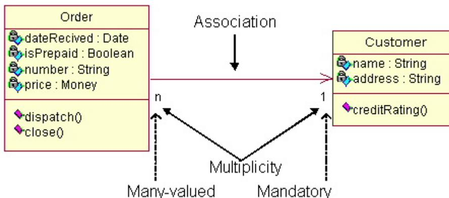
The association relationship is the most common relationship in a class diagram. The association shows the relationship between instances of classes. For example, the class Order is associated with the class Customer. The multiplicity of the association denotes the number of objects that can
